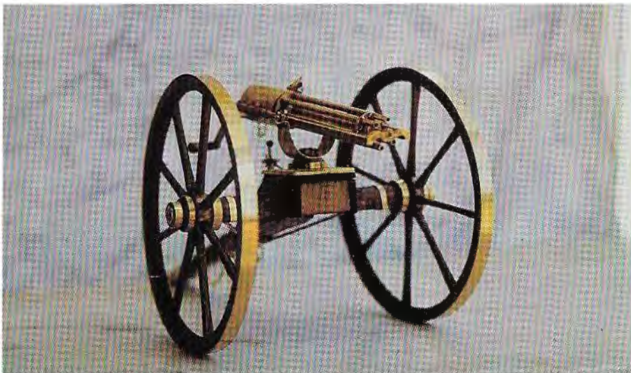
1862 Gatling Gun. Working crank, rotating barrels, cartridges and clip.
